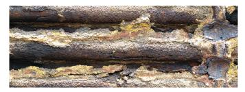
Due to its nature, calcium carbonate is soluble in cold water but will precipitate in hot water or hot surfaces. The bone like material will deposit itself on surfaces of equipment like cooling water pipes, shell side of a shell-and-tube heat exchanger and other cooling equipment. Every millimetre of calcium coating on a shell-and-tube, means resistance for heat transfer and the need for more cooling water, leading to higher pumping costs.
