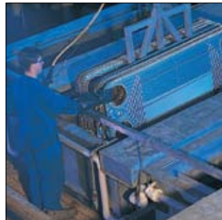
Chemical cleaning of plates in heated, agitated tanks. Ensures a clean, deposit-free metal surface.
