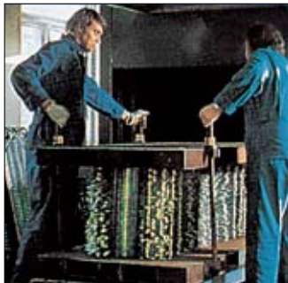
Special 2-component epoxy gluing, followed by an oven cure for the strongest bond, provides longer gasket service life.
