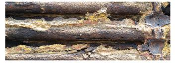
Due to its nature, Calcium Chloride is soluble in cold water but will precipitate in hot water or hot surfaces. The bone like material will deposit itself on surfaces of equipment like cooling water pipes, shell side of a shell and tube heat exchanger and other cooling equipment. Every milimeter of calcium coating on a shell and tube, means resistance for heat transfer and the need for more cooling water, leading to higher pumping costs.
